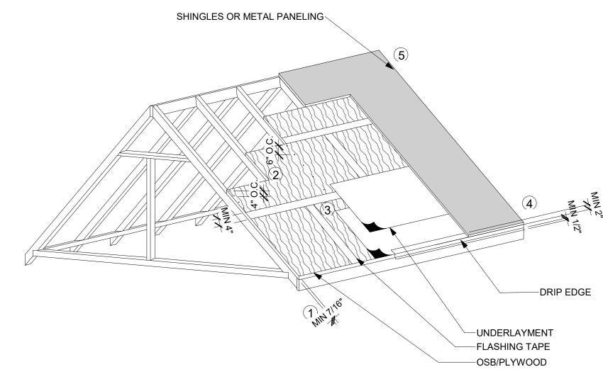
1. ROOF DECK THICKNESS REQUIRED TO BE MIN. 7/16 IN. OSB OR PLYWOOD.
