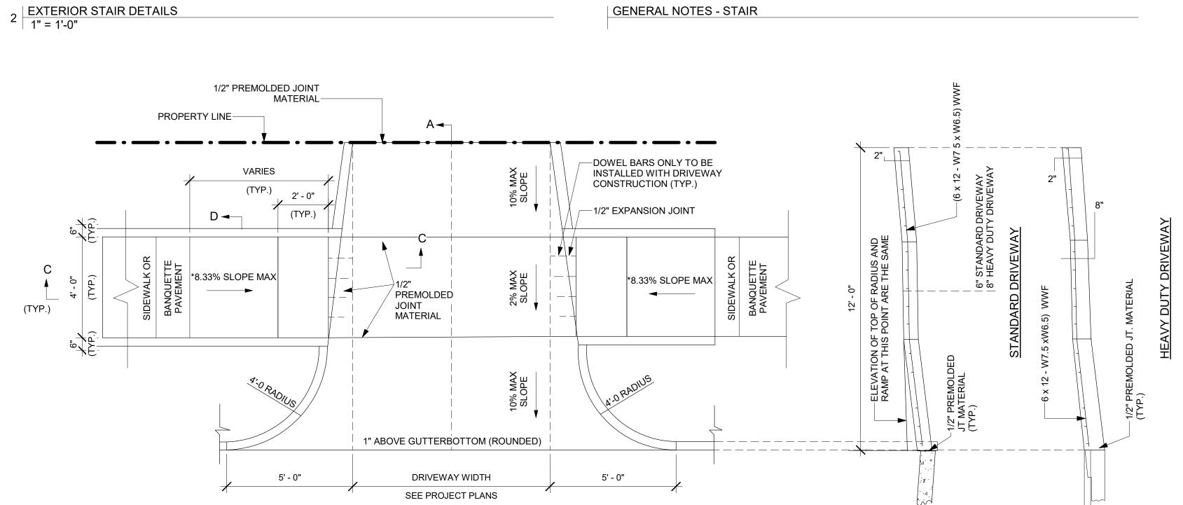
DETAIL OF STANDARD DRIVEWAY FOR CONCRETE VERTICAL CURB
